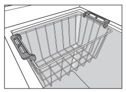
Position the baskets by hooking the handles onto the rim of the freezer.
